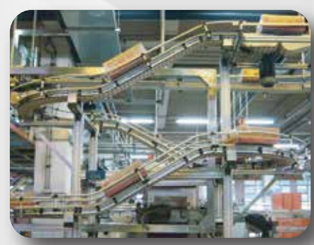
3-Dimensional Layout MODU conveyors make the most out of limited factory space by utilizing overhead space and small radius turns.
