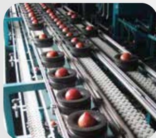
Puck system for fruit sorting line
