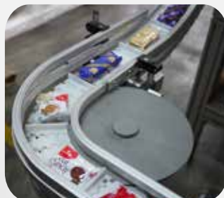
Cleated conveyor for biscuit packaging
