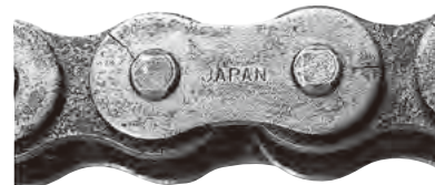
Fig. 32 Hydrogen embrittlement cracking
