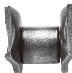
③ Offset link plate fatigue
