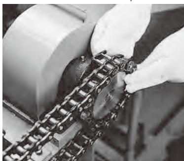
Fig. 8 Connecting on a sprocket
