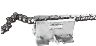
Fig. 3 Setting the roller chain in the chain vise
