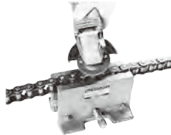
Fig. 2 Grinding the pin ends
