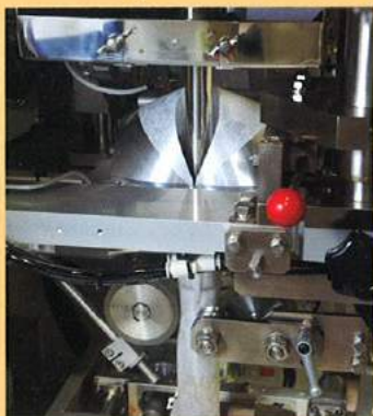
Longitudinal seal/cutting of the string filter
